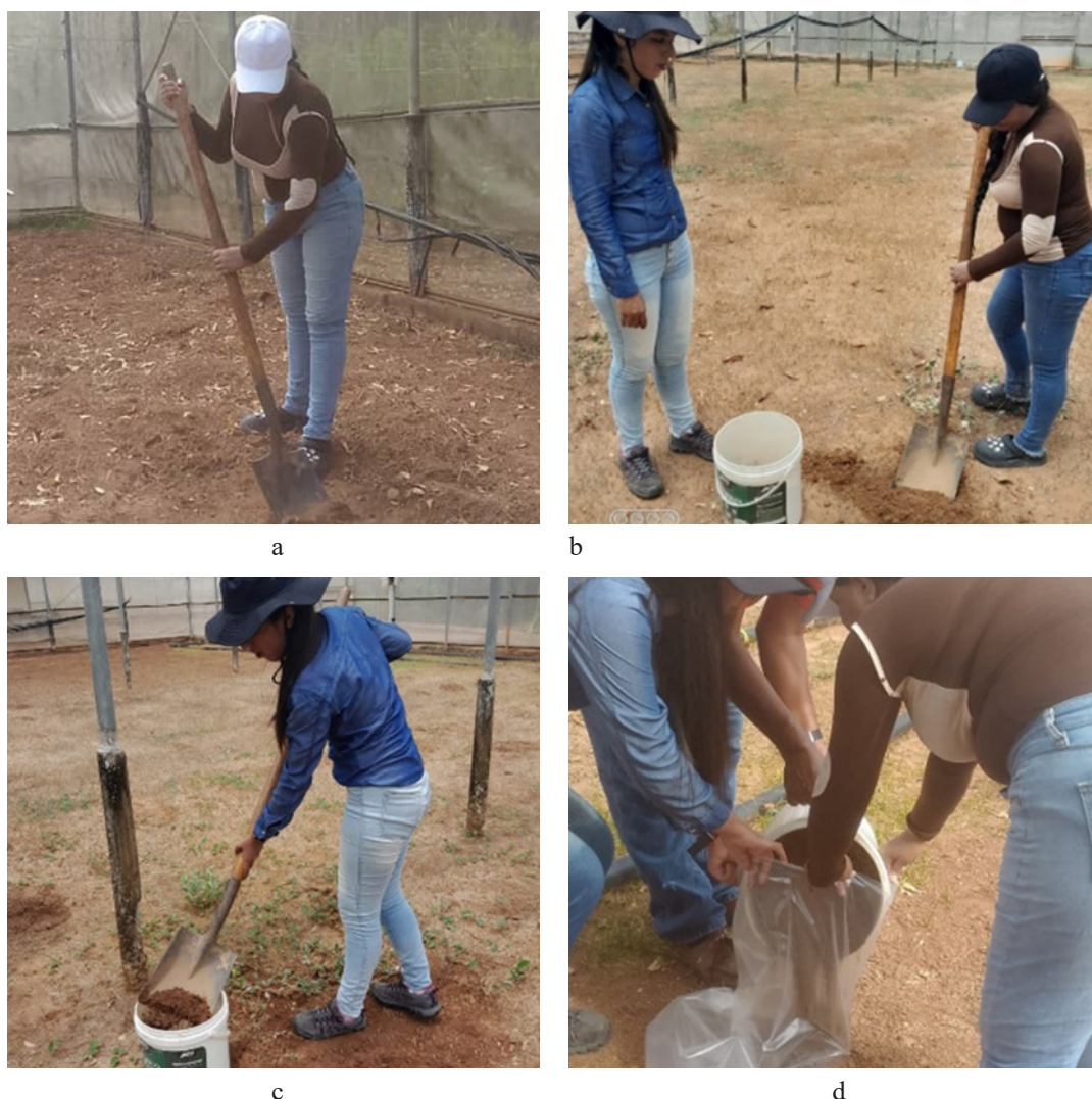
Figure 3. Sample collection a) removal of the vegetation layer, b) test pits, c) samples collected in a plastic bucket, d) transferred to a plastic bag
