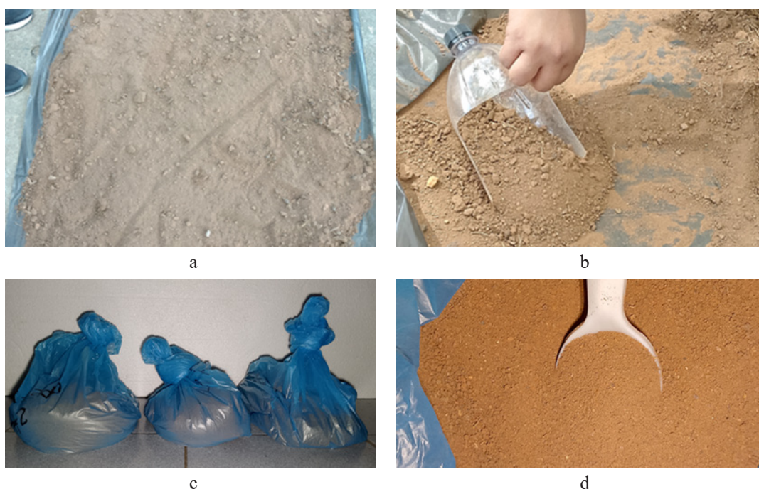
Figure 4. Sample preparation: a) homogenization and quartering, b) discarding of two quartering fractions, c) portion of approximately one kilogram, and d) sieved sample
